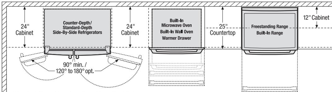
When installing refrigerator adjacent to wall, cabinet or another appliance that extends beyond front edge of unit, 20" minimum clearance recommended to allow for optimum 120° to 180° door swing, providing complete drawer/crisper access and removal.
