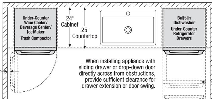
When installing appliance with sliding drawer or drop-down door directly across from obstructions, provide sufficient clearance for drawer extension or door swing.
