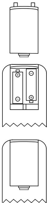
**NOTE:** When replacing batteries, it always a good idea to replace both at the same time. When the remote will not be used for an extended period of time, it is also a good idea to remove the batteries to avoid the possibility of damage due to corrosion. Batteries contain chemical substances and we recommend that you dispose of them properly and in compliance with any local regulations.
