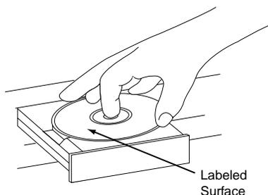
To close the drawer, press the appropriate **Open/Close button 7 14 3 30** or gently press on the outside of the front cover of the disc tray. When the drawer is closed the word **CLOSE** will appear momentarily in the **Information Display K**, and the letters **TOC** will begin to flash in the display once the drawer is completely closed.
