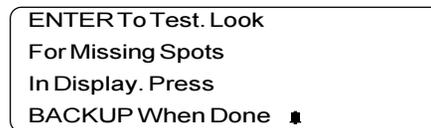
The Display Test Screen is shown below. Look for pixels that are not black. In other words, look for missing spots in the solid black characters. Press the BACKUP key to return to the Tool Self Test Menu when
