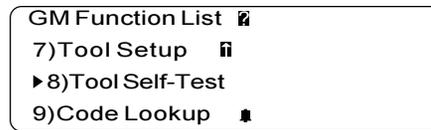
To select Tool Self-Tests on either screen, use the UP and DOWN arrow keys to move the cursor so it is pointing to the Tool Self-Tests option, then push the ENTER key to select this option.
