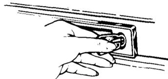
To lock or unlock the freezer you must hold the key in the lock while turning. The lock is spring loaded so the key cannot be left in the lock.
