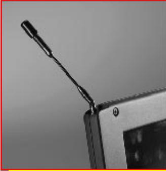
The laptop is equipped with a H.O.T. Antenna (High-gain, Omni-directional, Telescopic). The antenna is retractable\*, into the LCD assembly, and may swivel 360° for ease of use and increasing signal reception strength. Position the antenna to radiate away from the body to increase effective coverage.
