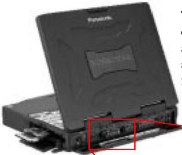
The laptop is equipped with an external antenna connector. An external antenna (i.e. mounted on a vehicle) may be connected to provide higher signal strength in fringe or low signal areas to maximize effective coverage.
