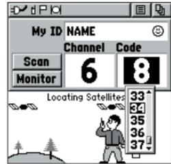
*Choose from 38 squelch codes. Setting the unit to zero will allow you to hear all transmissions on that channel, but you must be on the same code to radio back.*
