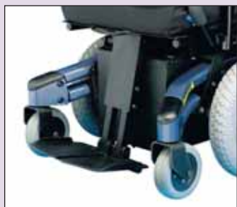
Center mount rigging provides excellent 90° foot positioning for tight hamstrings.
