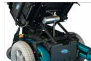
The actuator is integrated into the base and can be easily removed for battery servicing.
