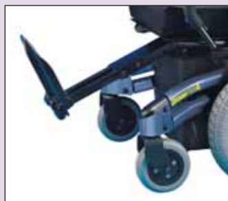
Allows for in-the-field knee angle adjustment from 90° to 60°.
