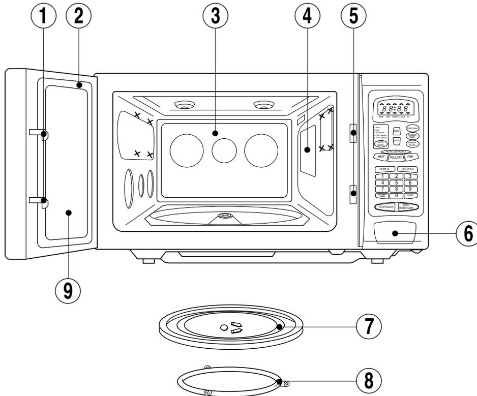
**1. Door latch** - When the door is closed it will automatically lock shut. If the door is opened while the oven is operating, the magnetron will automatically shut off.
