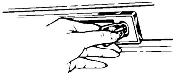
To lock or unlock the freezer you must hold the key in the lock while turning. The lock is spring loaded so the key cannot be left in the lock.
