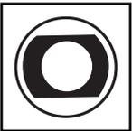
**Input Breaker (SMX1500SLT):** Protect your electrical circuit from overcurrent draw from the UPS load. If this breaker trips, remove some of the load, then reset by pressing the breaker in.
