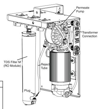
IMPORTANT: Remove white plug from module and insert black tube as shown. Insert RO module into filter head and rotate 1/4 turn until it stops. The label should face the front.
