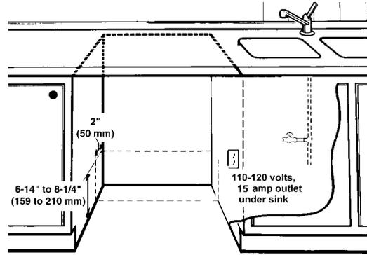
There should be an opening through the partition between the opening for the dishwasher and the area under the sink that is large enough for the power cord to pass through. This opening should not be more than 1-1/2" (38 mm) in diameter and the edges should be smooth and rounded. If the partition is metal it should be covered with an edge protector provided for this purpose by the manufacturer.
