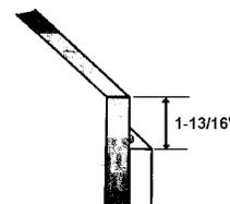
With this installation, the custom panel extends 1-13/16" inches above the dishwasher control panel, as illustrated.
