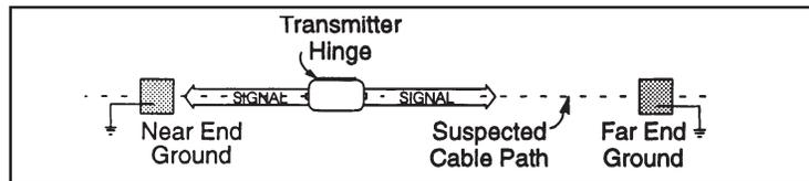
Place the transmitter on the ground over the target cable with the lid hinge in line with the cable path. Press
