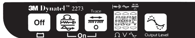
To test the Batteries, press and hold
