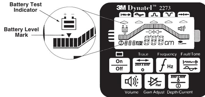
The Receiver batteries are tested for two seconds every time the unit is turned on. The time interval can be extended by pressing and holding
