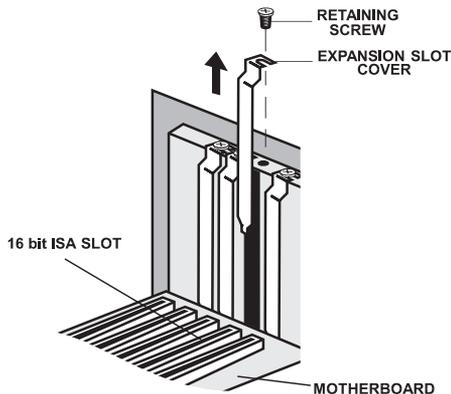
**Figure 2: Removing the Backplate**
