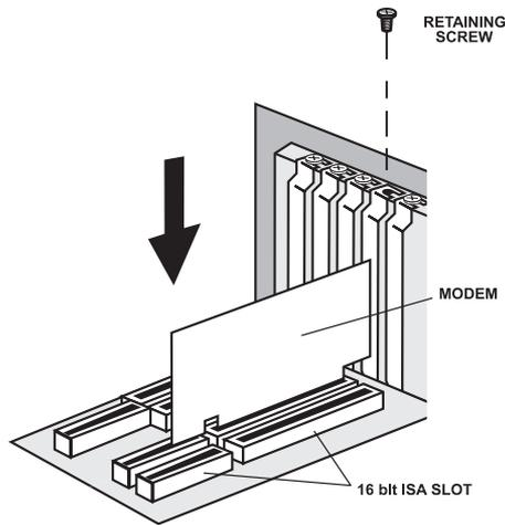
**Figure 3: Installing The Modem**
